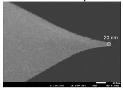
Platinum silicide probes. Advantages: small radius, excellent conductivity, good wear-out behavior
