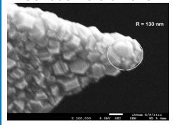
Conductive diamond probes. Advantages: hard, long-lasting coating. Disadvantages: large radius, low conductivity
