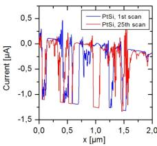
Cross sections of current images of (a) a commercial Pt probe (Pt, left image) and (b) a PtSi probe (PtSi, right image). TUNA mode, DI Icon, sample bias -0.25V, force  $1\mu$ N, total tip travel distance 13mm. For each tip a cross section out of the first and the last scan is shown.
