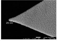
Platinum(Iridium) coated probes. Advantages: relatively small radius, excellent conductivity. Disadvantages: fast wear-out
